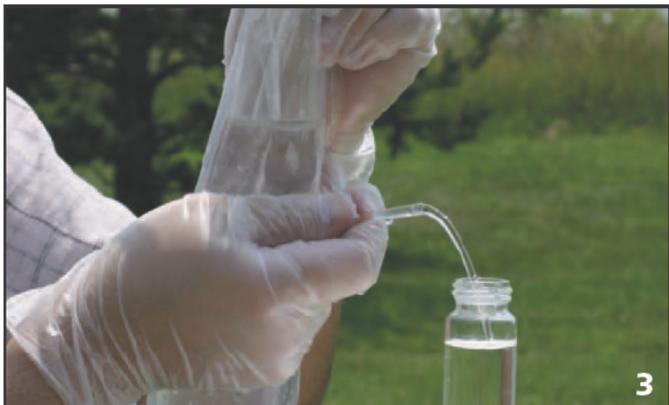
Discharge the sample into the desired container. (Photo 3, bottom left)
