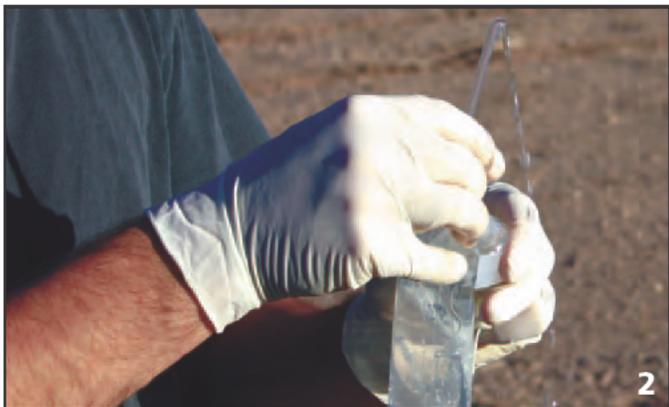
Then, push the pointed discharge tube through the outer polyethylene sleeve about 3-4 inches below the white reinforcing strips. (Photo 2, middle left)
