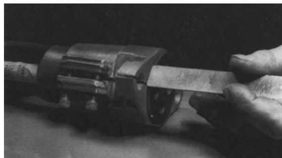
Figure 22 Checking gap, terminal box clamp to terminal box
