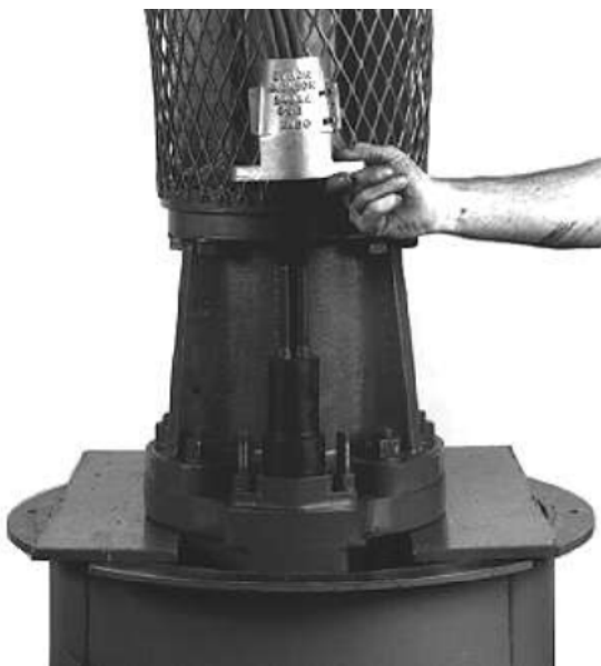
Figure 24 Terminal box installed
