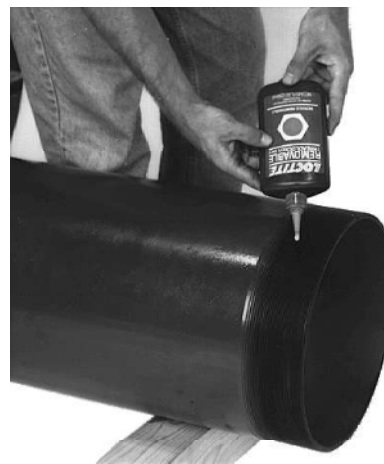
Figure 14 Applying thread locking fluid
