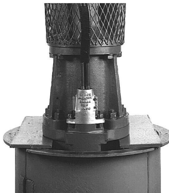
Figure 25 Power cable clamp installed
