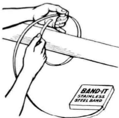
Figure 29 Use of "Band-It" steel band, step 1
