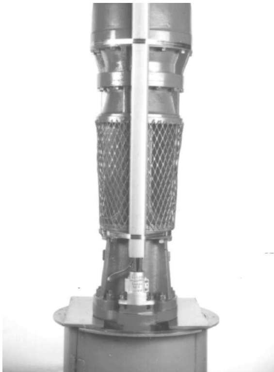
Figure 28 Outer guard and band in place - example
