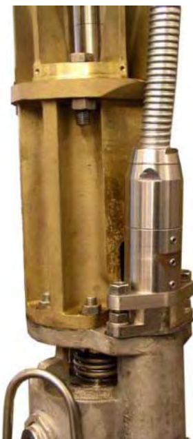
Figure 26 Metal housing power terminal connector (4 000 V-cable)
