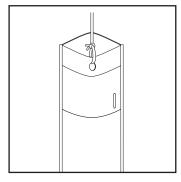
Attach line to hole at top of HydraSleeve.
