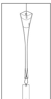
Sampler is ready to insert into the well.
